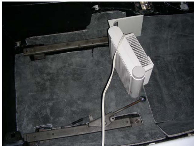
Figure 9. Like-original padding installed in the passenger seat compartment with rails mounted to check proper fit. Note the small heater that I used to warm the area while the glue dried (it was still a bit like winter outside).
