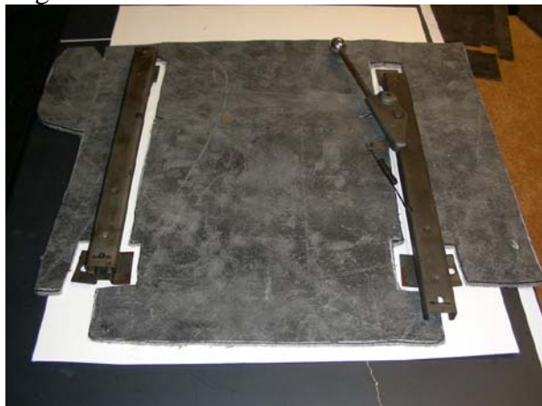
Figure 8. I removed the passenger seat rails from the seat and used them to check the padding and make sure that all of the stock cuts fit properly. Some minor adjustments were needed in this padding for a "perfect" fit.
