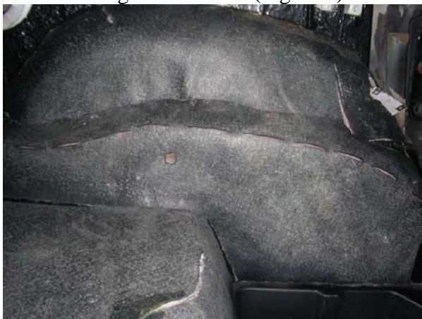
Figure 7. Like original padding installed over the rear driver's wheel well and rear storage deck. Notice the serrated cuts that I made in the heavy padding to follow the contours of the wheel well and make installation easier. I got this idea from the "original padding" that I removed from the car, which had similar cuts. After initial installation of the padding, I discovered that I needed to remove significantly more material around the shoulder
