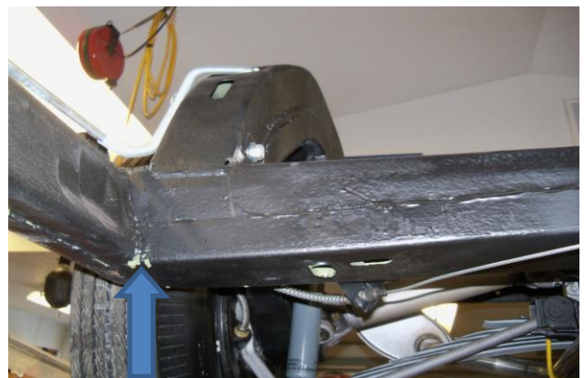
63 to around 17000 of 64 had no rear corner braces
