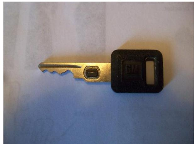
VATS stands for Vehicle Anti-theft System. Each VATS key has a resistor embedded within the key blade, and each resistor has 1 of 15 possible values. Decoding a VATS key is very simple, but it requires you know how to use an ohm meter.
