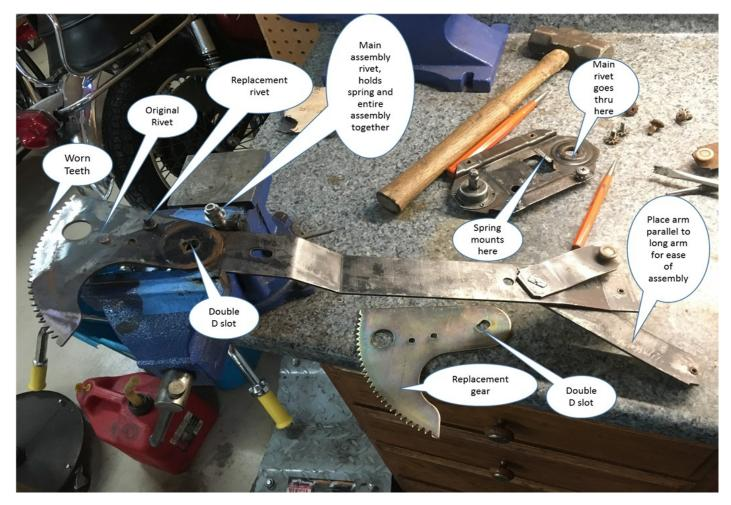
This is my original passenger side manual window regulator, the rivets were ground off....you can see remnants of dip paint process in black.
