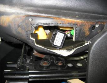
Replace the switch, reassembly is the opposite of removal. I tested the switch before I reassembled. Screw the switch in place. Put the cover back on
