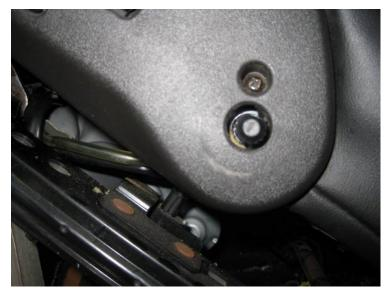
Once the plastic panel is off you will see a metal panel with three screws. Remove them and remove the panel, it is what retains the switch in the mounting hole.
