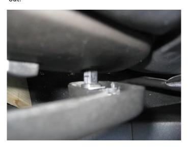
The plastic side panel of the seat is now free. From the back of the seat pull it away. It is tucked behind a metal rail on the top edge, so pull up slightly as you pull away. At the front edge of the seat there is a tab that retains the panel. Once the rear and top of the panel are free pull towards the front of the car to release the panel completely. Let it hang, no need to remove it completely.
