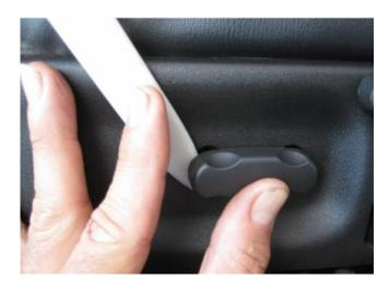
Remove power seat switch by gently prying it away from the seat with a non-marring tool. I use a nylon pry bar. Pry from each side until the pressure clips release.
