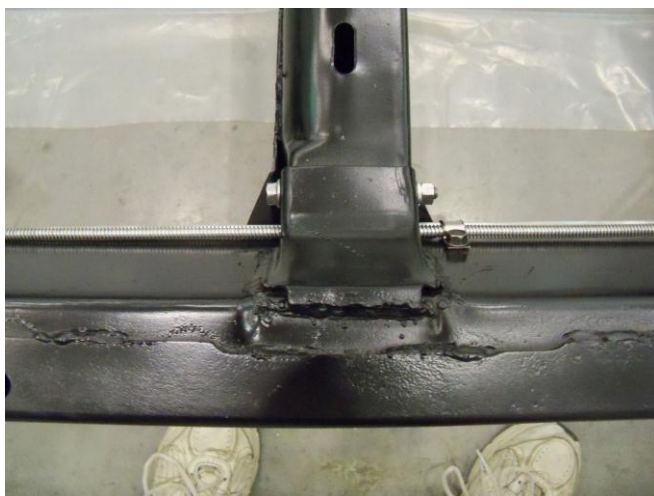
1968-1979 cars with Automatic had bolted cross members.
