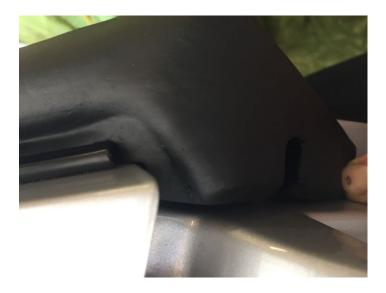
Once you have both sides in place and there are no gaps and the strip is not stretched out, you can begin to place adhesive. Gently remove one side at a time and place adhesive directly on the weatherstrip. The bottom of the weatherstrip is the only places you will apply adhesive directly to the strip. All other places you will apply adhesive into the strip channel.
