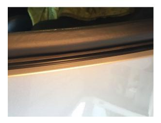
• You want to make sure you position the new weatherstip flush to the B Pillar support and place in both side channels to ensure one side is not longer than the other and there are no gaps. The weatherstip has a notch at both ends so you can align the bottom to the frame.
