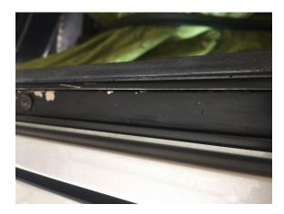
• Once all the adhesive is removed, place the new weatherstrip in the SIDE channels ONLY. DO NOT GLUE weatherstip at this time.
