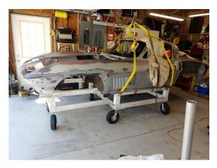
Removing the body again so I can finish replacing body mounts and prepping the underside.
