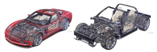
The C6 was more evolutionary than revolutionary. The suspension was mostly the same, with some tweaking that resulted in better on-center steering feel. Chassis specs were similar, with C5 advances like the transverse leaf springs, balsa wood floor construction and hydroformed side rails also part of the C6. As one can see in the two pictures that follow, the C6 was essentially the same highly regarded suspension as found on the C5.
