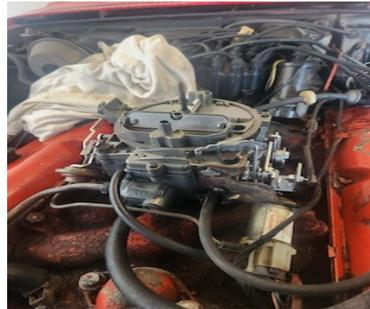
Once I got the carb back, it was an easy reinstall by using the newly provided gasket. Secured the carb back on with the four nuts and reattached the accelerator cable and choke spring coil. A little adjusting of the carb with the help of Gus Tsamouras and others checked one vital thing off my list to keep my dad's car running and as original as possible. **JOB WELL DONE!!!!**
