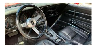
The final horn button and lock ring configuration is shown in the photo of the Corvette with a brown interior. Note that both the horn button and lock ring are the same color as the steering column.
