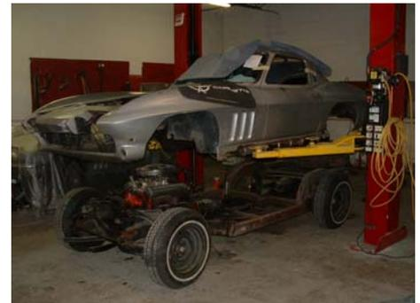
how bad the frame was until he had the body off the car. At that point, he discovered the inside frame rails were also rusted and much time was spent getting the frame right before dipping and
