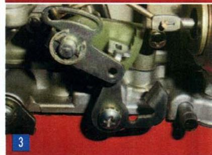
1 The greenish-hued plastic fast idle cam (behind the choke operating lever in the foreground) is pivoted all the way down with the engine warm and the tang on the primary throttle lever is clear of the top of the cam.
