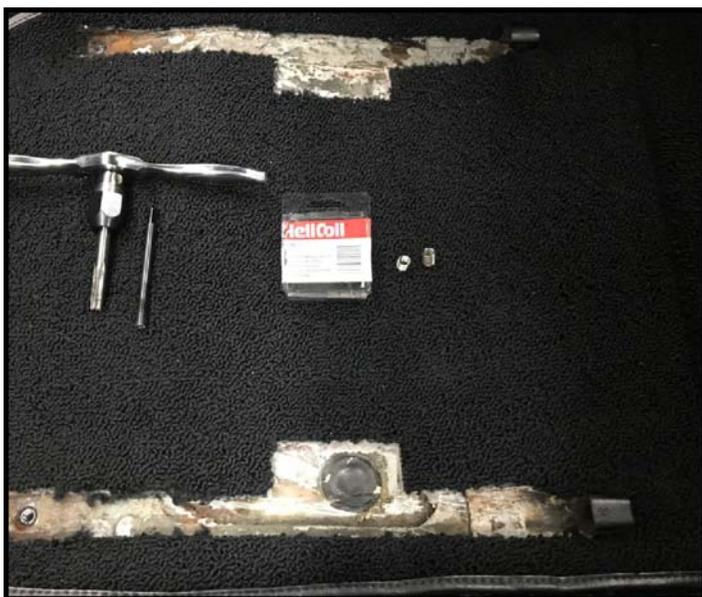
Helicoil inserts in all four seat mounting locations. You can see the installed Helicoils in the picture. I then mounted the seats and replaced the original screws. Once the seat and screws are installed this is an undetectable repair.
