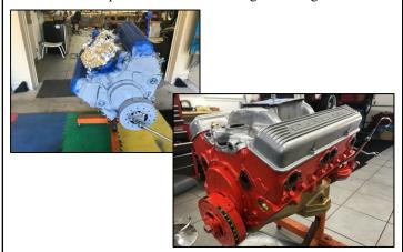
After the engine was painted, we installed a new oil impregnated crank pilot bushing, a lightweight 15 pound, L-88 (GM) flywheel with a McLeod performance clutch assembly and a Lakewood
