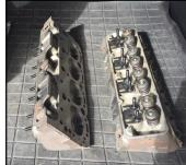
HD pushrods were installed. Low profile locking rocker arm nuts with extra thick valve cover gaskets were used to clear the stock aluminum Corvette valve covers for that nostalgia look.
