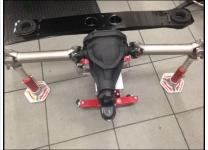
Tulsa. A new 3.73:1 ring and pinion was installed in place of the 3.31:1 gear during the rebuild. The trailing arms were also rebuilt by V-Tech Corvettes in Rockford, Ill.. I added a <sup>3</sup>/<sub>4</sub>-inch anti-roll
