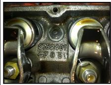
Left Head Casting Number: 3782461 327CI 350HP for 1966 with 2.02 intake and 1.60 exhaust valves
