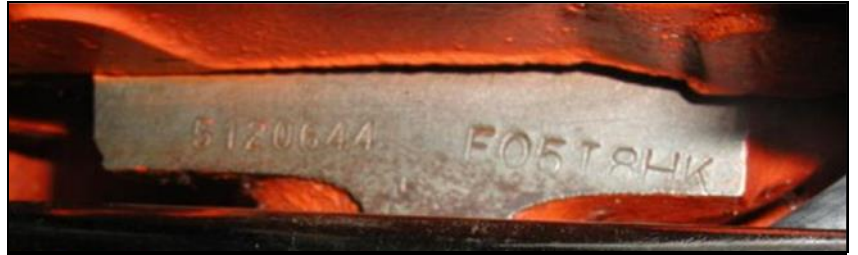
Photo of rare 1965 engine pad with the 365hp solid lifter engine and air conditioning. Note the crooked F0518HK engine stamp. Many "Original" 365hp air cars in 1964 and 1965 have similar stamps, that is they are crooked. Perhaps the AC mounting bracket was on the engine when the stamp was applied.
