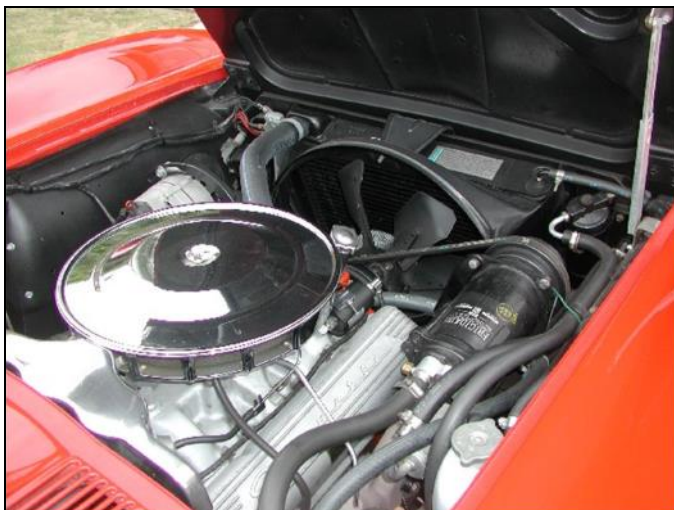
The photo below shows the extra plumbing on K-19 Cal Smog cars with air conditioning. One has to remove the R/F tire and gain access thru the inner fender rubber flap to remove the # 2 and # 4 spark plugs when doing a tune up.
