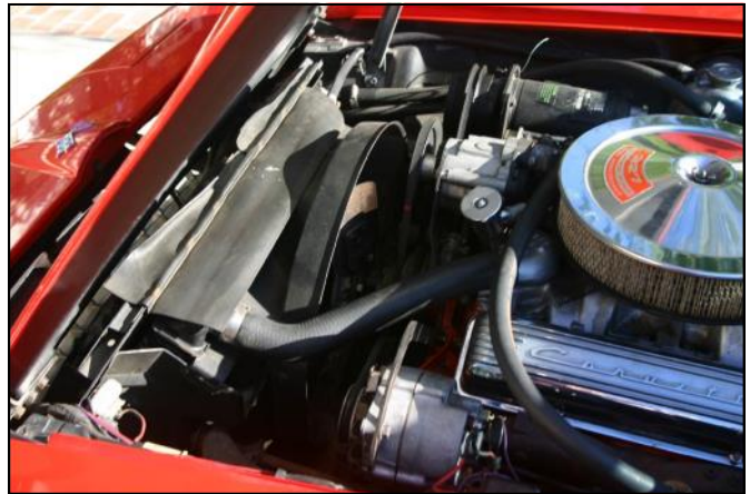
Note the extra rubber insulation around the radiator. All small block air cars had this to help with forcing more air thru the radiator for overheating problems
