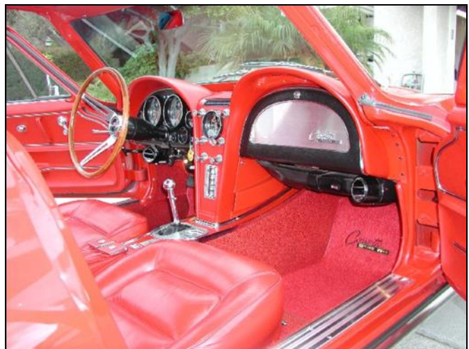
Inside air ducts in the center dash, and one each under the right and left dash supply cold air to the interior.
