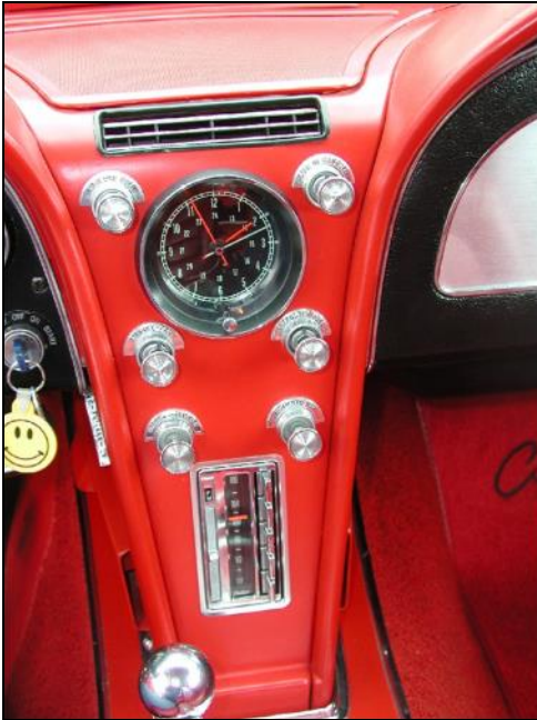
A center duct AC thermometer will read 34 degrees on a good running AC System
